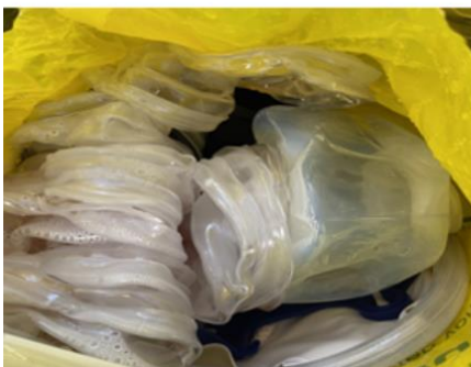
Once removed, a large glomerulus of melted, intertwined material was observed which required a scissors to cut out as the autoclave bag was adhered to it.
