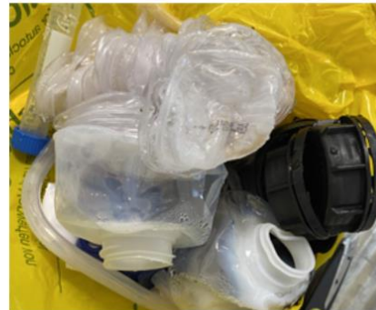
Once the bag was cut open you can visibly see the conjoined material and also the black caps and catheter which did not melt.
