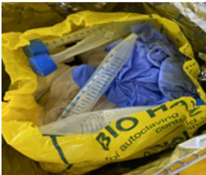
Once removed, a large glomerulus of melted, intertwined material was observed which required a scissors to cut out as the autoclave bag was adhered to it.
