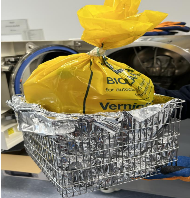
Figure 4 - Autoclave loaded with wire rack to contain potential leakages
