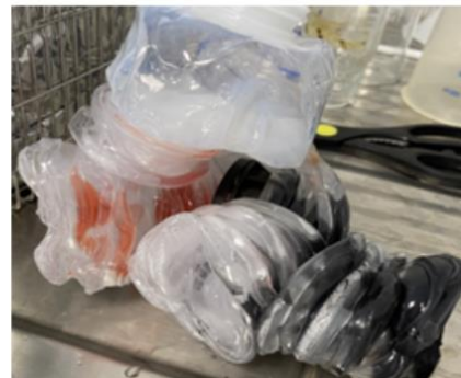
The glomerulus upon further inspection had melted around various different materials which were used during the trial
